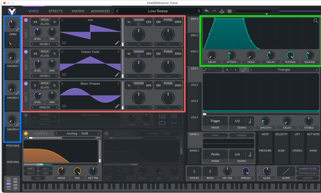
Figure 3.5. Screenshot of the Vital Synthesizer plugin. On the left border, user definable “Macro” dials are highlighted in blue. On the left side marked in red, three active oscillator curves are shown. In the top right green highlighted window, the ADSR envelope for oscillator one is pictured.
